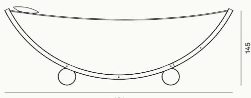
Galvanized steel base and wooden structure hammock /
