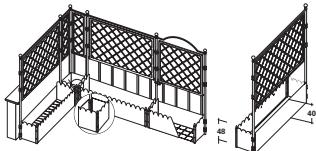
Wall-mounted Solaire planters must only be used with posts, grilles and the other accessories suggested on these and previous pages. 4 aluminium couplings Ref. G33NC, are necessary for fixing to posts, making the length of the planters 37, 109, 157 e 181 cm and respectively compatible with 30, 102, 150 e 174 cm grilles. A 42.5 x 42.5 cm corner unit is also available.
